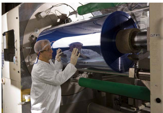
Figure 4: Konarka roll to roll manufacturing process, illustrating the compatibility with mass production.
